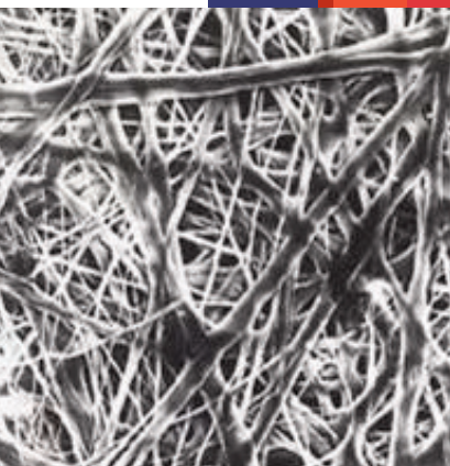
Even particles less than 1 micron in size can't pass through Tyvek® fabric.
